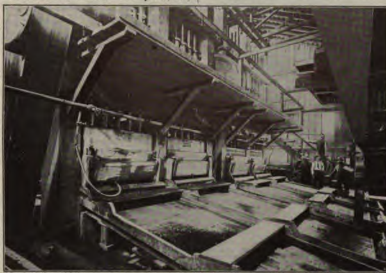
Much of the gold dug from mines is embedded in hard rock. This rock is broken up into small pieces which are crushed into powder in a "stamping mill." The stamps are immense pestles, weighing over 1,000 pounds, which are raised by machinery and are dropped upon the rock, crushing it into powder. Flowing water washes the powdered rock over copper plates covered with quicksilver, to which most of the gold adheres, while the sand is washed on to the boxes which you can see at the end of the plates. The quicksilver is evaporated, leaving the pure gold. Some gold is left in the sand and is taken out by a process called "concentration."
